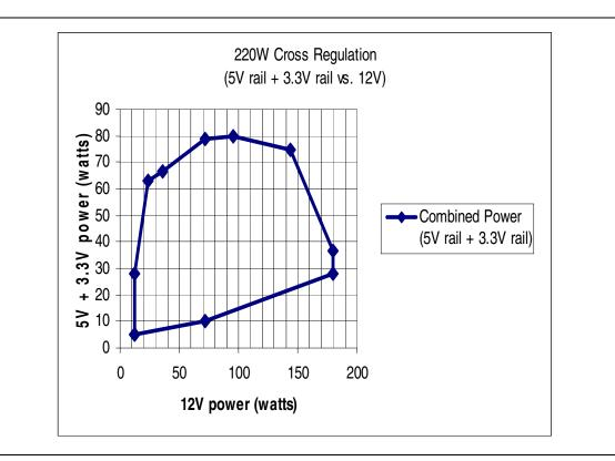
Figure 3. Cross Loading Graph for 220W Configuration
